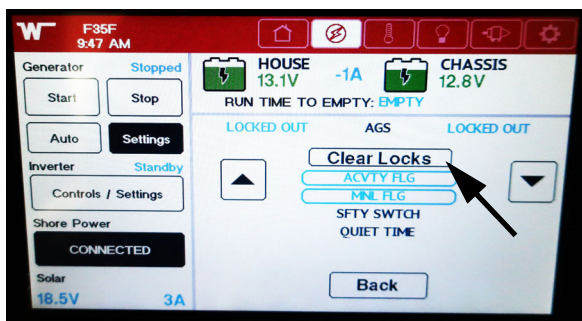
On this screen use the "Clear Locks" button to clear any conditions that automatically disabled the Auto operation settings, such as the vehicle being started and moved. Any previous or new settings can be enabled once the vehicle is parked and in a safe location. -Typical View
