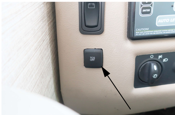
Traction Control Button is located on the driver side left of the headlight switch -Typical View
