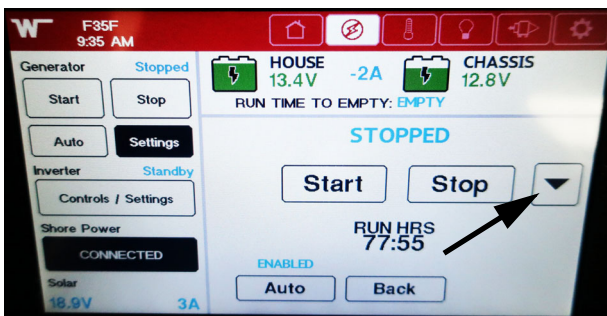
Select the down arrow to view the next screen. -Typical View
