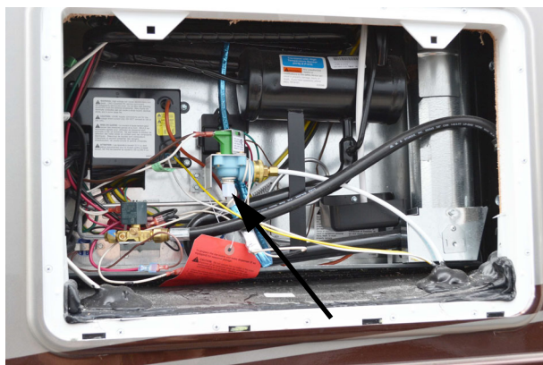
Ice Maker Water Supply Connection (Located in refrigerator service access compartment on outside of the motorhome) -Typical View
