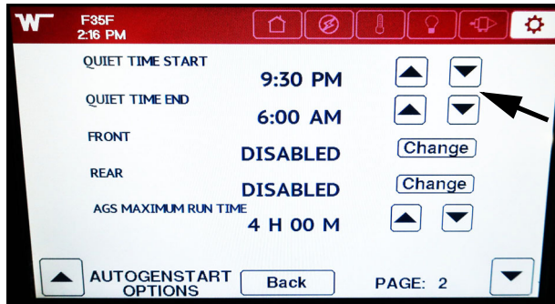
Page 2 of the AGS shows the quiet time start and end settings (local time is used to prohibit starting the genset during quiet time settings). -Typical View
