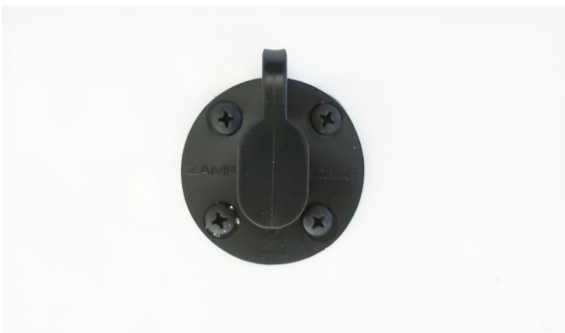
Single Solar Port (Located inside driver side exterior compartment-typical view)
