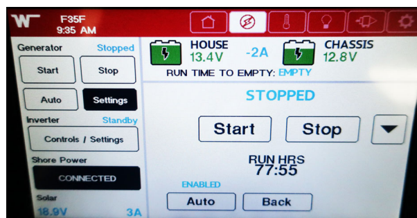
Generator Settings Screen Use this screen to customize various triggers to automatically start and stop the generator. Select the down arrow for further customizations and options. The total run hours are also displayed on this screen -Typical View
